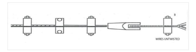
6. Place a special clamp 'B' at the end of the serving (clamp is bored to fit over serving). Open out the wires to form a brush and clean thoroughly with Trichloroethylene (TCE) or other suitable degreasing solvent. Petrol or paraffin is not recommended.
